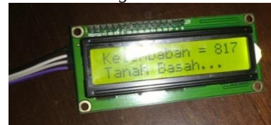
Gambar 7 Keadaan LCD saat sensor berhasil ter-setting
